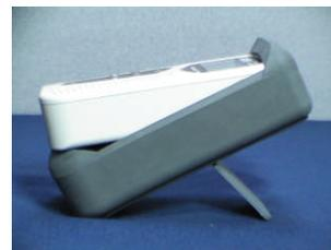
The conductivity meter can be pushed out of its rubber boot.
